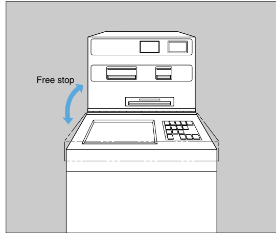
For opening/closing of maintenance machine doors.
